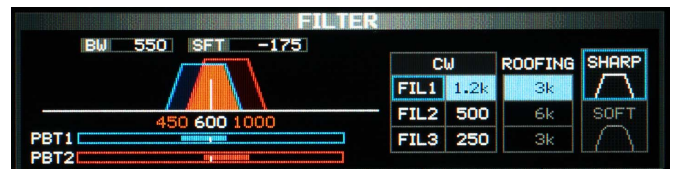
Digital IF filter setting example
